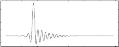
A waveform plot showing a sharp initial peak followed by a series of smaller, decaying oscillations, characteristic of a minimum phase filter.                                                    |
