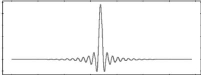
A waveform plot showing a sharp peak with significant pre-ringing (oscillations before the main peak) and post-ringing (oscillations after the main peak), characteristic of a brick wall filter. |
